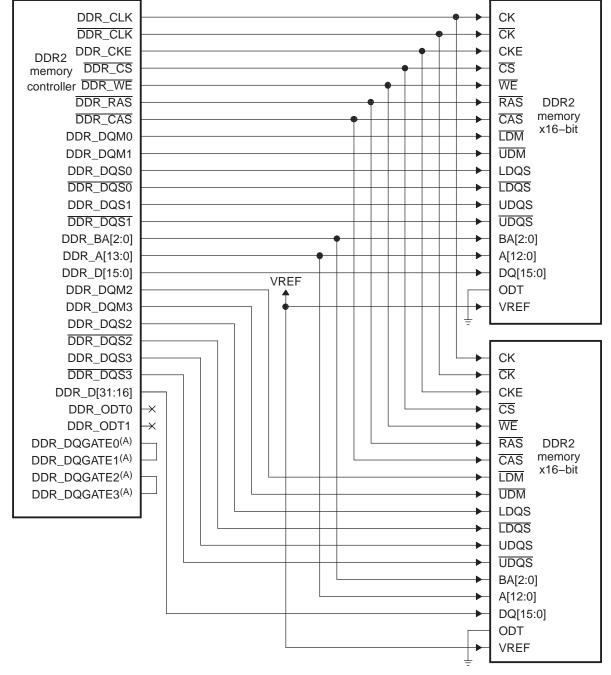
Figure 17. Connecting to Two 16-Bit DDR2 SDRAM Devices
